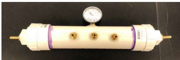
Supplementary Figure S4. Manifold with a pressure gauge to facilitate the simultaneous collection of three samples of airborne pathogens.
