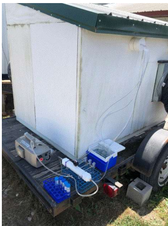
Supplementary Figure S12. Pathogen sampling system before the MERV filtration unit samples raw exhaust from swine barn fan.
