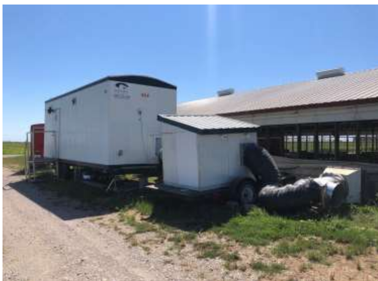
Supplementary Figure S10. Mobile laboratory for UV and filtration treatment deployed for testing mitigation of gaseous emissions at a swine farm.
