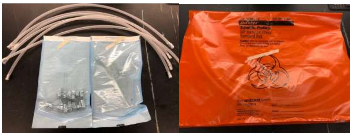
Supplementary Figure S15. Sterilization of impingers, air sampling tubing, and the impinger-tube connectors prepared for autoclaving.
