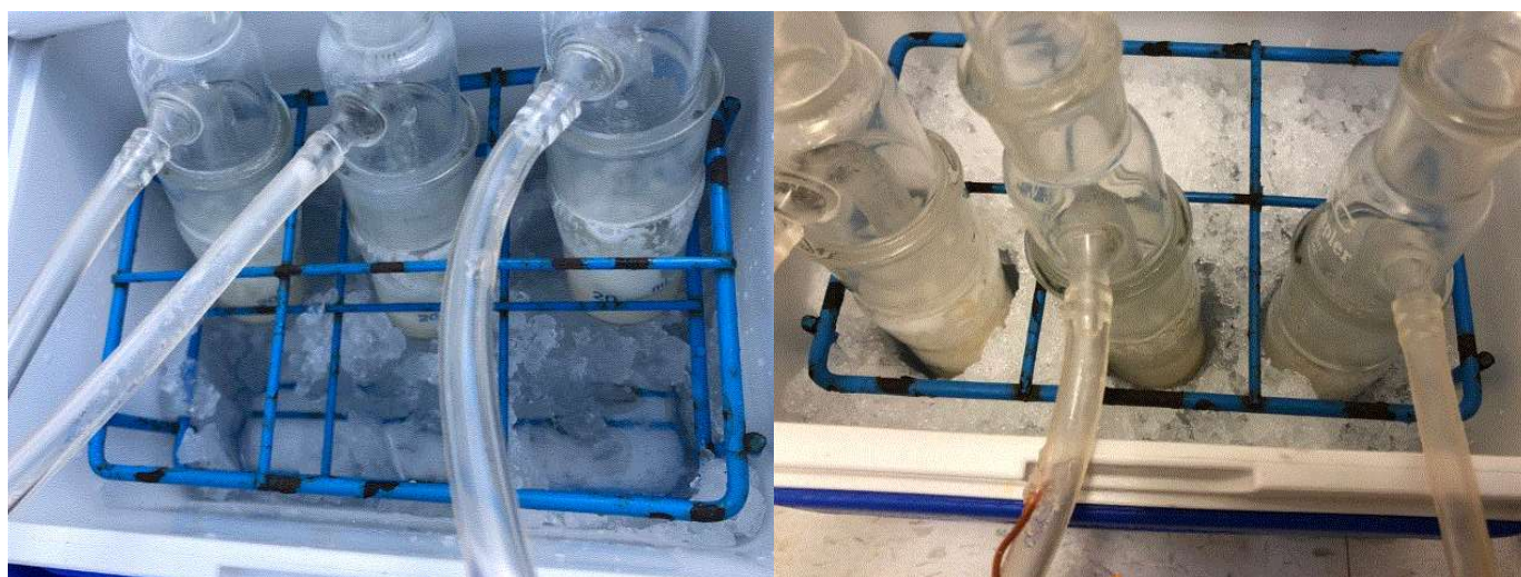
Supplementary Figure S7. Effects of the antifoaming agent addition into impinger solution. Foam formation during sampling (Left); No foam formed when Antifoam A added (Right). Impingers were held in an ice bath during air sampling.
