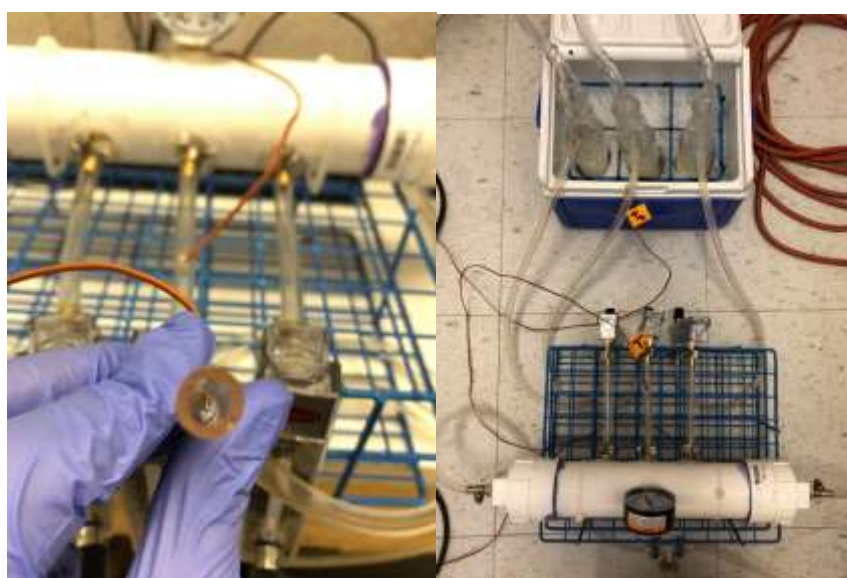
Supplementary Figure S9. Air sample temperature monitoring. (Left) thermocouple tip and seal; (Right) thermocouples installed immediately downstream from the impinger and after airflow monitor (rotameter).
