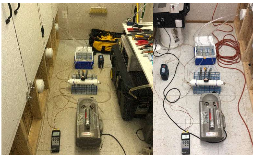
Supplementary Figure S8. Airborne pathogen sampling system. (Left) Air inlet to the UV mobile lab (downstream from the MERV filtration unit); (Right) air outlet after UV treatment.
