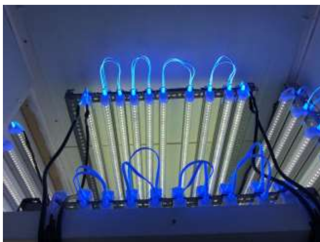
Supplementary Figure S11. Arrangement of 55 UV-A LED lamps installed in one of the chambers inside the mobile laboratory to treat emissions from the swine barn.
