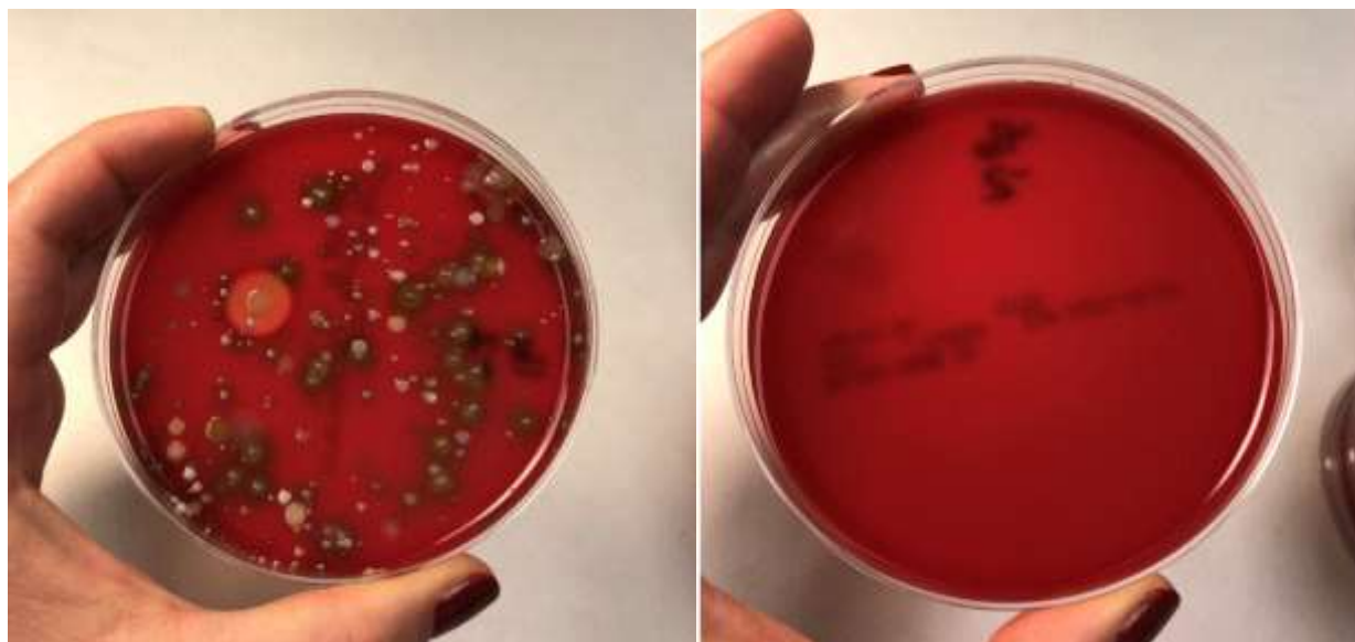
Supplementary Figure S13. Colony-forming in the culture medium after sampling for 60 min. (Left: before MERV filtration, Right: after MERV 8 and 15 filtration).
